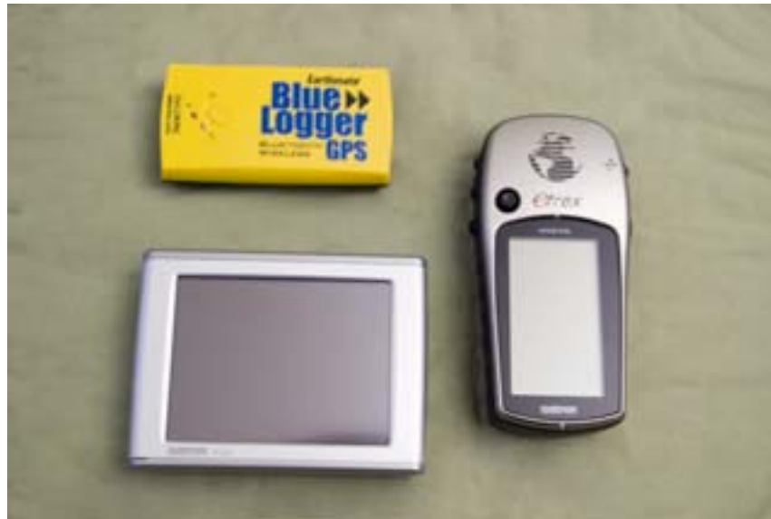
Figure 1: GPS receivers come in different shapes in sizes: GPS logger (top left), handheld GPS (right), vehicle nav system (bottom left)
